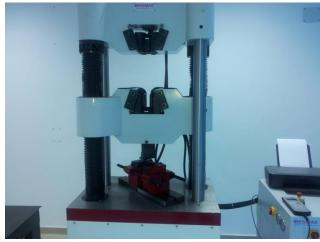
Mezan Company can perform tensile and bending tests of rebar and other metals (circular or rectangular shape)
